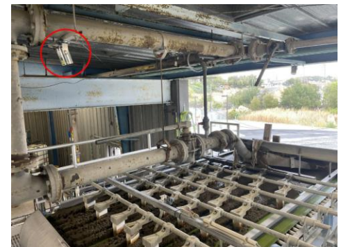
Figure 3: Waterproof camera mounted above the belt press using magnet.
